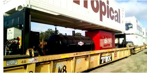
Provides reliable power for up to 10 containers under continuous operation and high ambient conditions. The unit is capable of supplying power to containers anywhere on the terminal or for double stack rail car operation. The unit is totally self-contained on a 40 ft. ISO steel flat rack which allows for easy handling for loading/unloading or for positioning on the ground.
