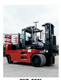
**XHC-600L**Rated Capacity 60,000-lbs. (27,216 kg) 36-in. (914 mm) Load Center 125-in. (3,175 mm) Wheelbase
