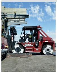
**TX-330SL**Rated Capacity 33,000-lbs. (14,980 kg)
