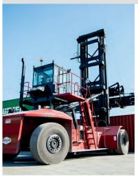
XLC-975 Rated Capacity At 97-in. (2,464 mm) Center of Load 90.000-lbs. (40.824 kg) / 2-high Stacking 80,000-lbs. (36,288 kg) / 5-high Stacking Rated Capacity At 106-in. (2,692 mm) Center of Load 82,000-lbs. (37,195 kg) / 2-high Stacking 75,000-lbs. (34,020 kg) / 5-high Stacking 236-in. (5,994 mm) Wheelbase
