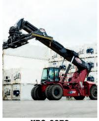
XRS-9972 Rated Container Capacity 99,000-lbs. (45 t) First R ow / 4-high Stacking 9.5-ft. (2.9 m) Rated Container Capacity 90,400-lbs. (41 t) First Row / 5-high Stacking 9.5-ft. (2.9 m) 258-in. (6,550 mm) Wheelbase
