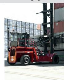
**XEC-205/6**Rated Capacity for 9.5-ft. (2.9 m) High Containers: 20,000-lbs. (9,072 kg) / 6-high Stacking Rated Capacity for 8.5-ft. (2.6 m) High Containers: 20,000-lbs. (9,072 kg) / 7-high Stacking 103-in. (2,616 mm) Load Center 180-in. (4,572 mm) Wheelbase
