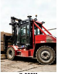
**X-360M**Rated Capacity 36,000-lbs. (16,330 kg) 24-in. (610 mm) Load Center 121-in. (3,073 mm) Wheelbase
