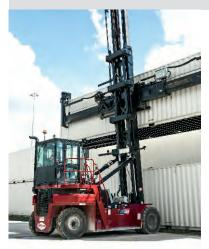
**XEC-155/6**Rated Capacity for 9.5-ft. (2.9 m) High Containers: 15,000-lbs. (6,804 kg) / 5-high Stacking Rated Capacity for 8.5-ft. (2.6 m) High Containers: 15,000-lbs. (6,804 kg) / 6-high Stacking 100-in. (2,540 mm) Load Center 150-in. (3,810 mm) Wheelbase
