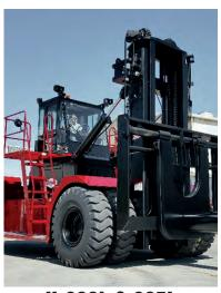
**X-800L & 925L**X-800L Rated Cap. 80,000-lbs. (36,287 kg)
