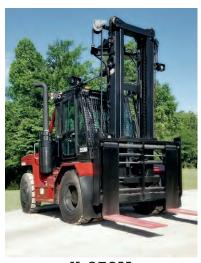
**X-250M**Rated Capacity 25,000-lbs. (11,350 kg) 24-in. (610 mm) Load Center 121-in. (3,073 mm) Wheelbase
