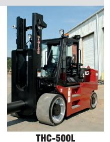
Rated Capacity 50,000-lbs. (22,680 kg) 30-in. (762 mm) Load Center 110-in. (2,794 mm) Wheelbase
